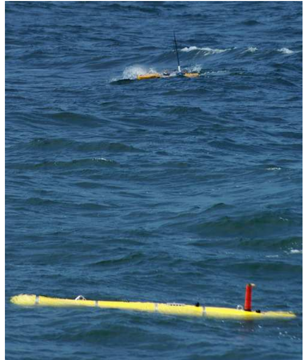
Fig. 1. An Autonomous Underwater Vehicle (AUV), here surfaced (foreground) uses an Autonomous Surface Craft (ASC) (background) as a navigation aid. The GPS-derived position of the ASC is obtained by the submerged AUV through an acoustic modem. Using time-stamped messages and globally synchronized clocks on all vehicles the AUV is also able to determine its range to the ASC through time-of-flight measurements.
