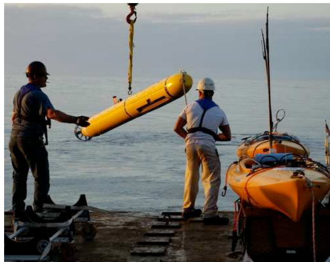
Fig. 1. An Autonomous Underwater Vehicle (AUV) on the crane and two Autonomous Surface Craft (ASC) on deck after a cooperative navigation experiment. The GPS-derived position of the ASCs is obtained by the submerged AUV through an acoustic modem. Using time-stamped messages and globally synchronized clocks on all vehicles the AUV is also able to determine its range to the ASC through time-of-flight measurements.
