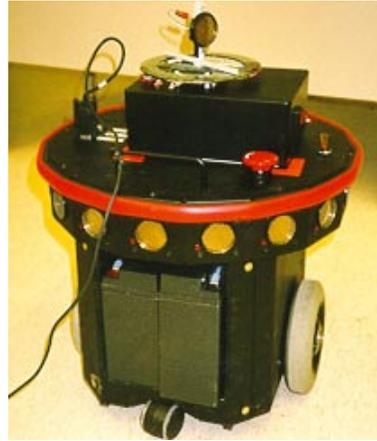
Figure 4: The Nomad Scout robot with the Polaroid ultrasonic sensor mounted on top.
