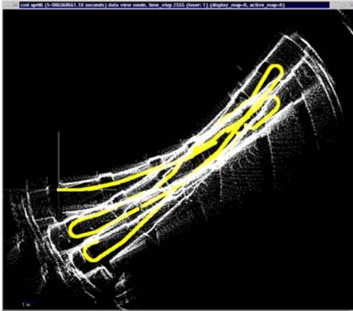
Figure 1: Laser data for a short corridor experiment, referenced to the dead-reckoning position estimate
