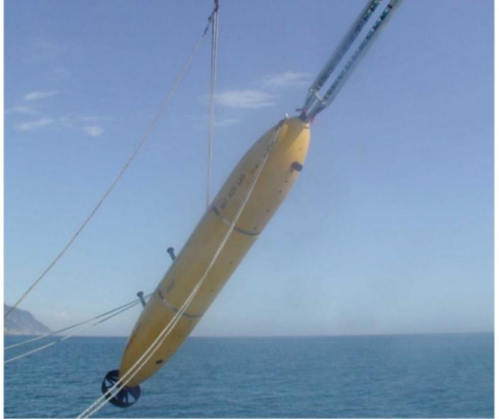
Figure 5: Caribou the MIT Department of Ocean Engineering’s AUV being launched in the GOATS 2002 Experiment near Italy. The forked “prong” structure at the front of the vehicle is a 16 element Synthetic Aperture Sonar (SAS).
