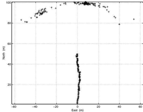
Figure 4: All vehicle and feature states that survive at least one pruning pass. 399 total states passed at least one cycle of pruning, 217 are feature states and 182 are vehicle states.
