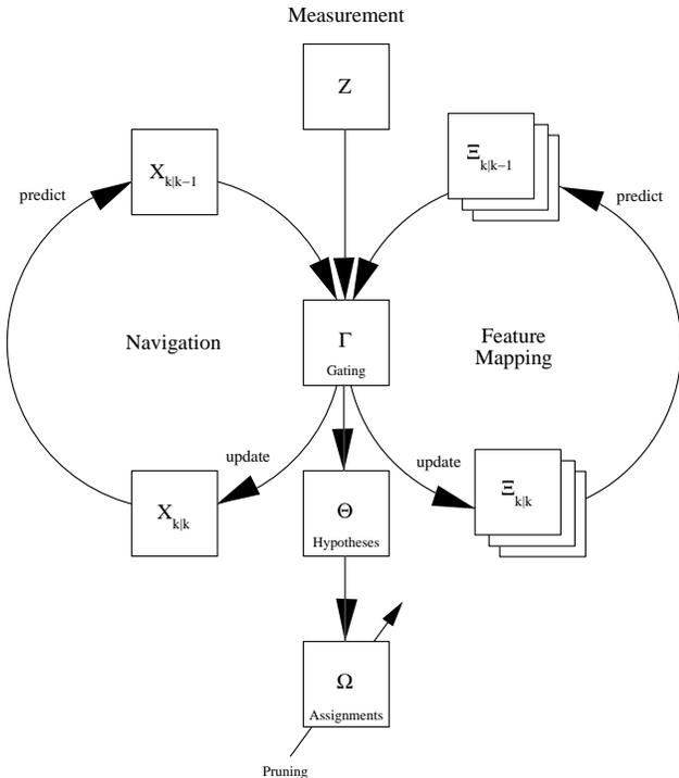
Figure 2: Process flow for MHCML. Information from relative measurements is used to update vehicle navigation and feature models simultaneously. Hypotheses and assignments are formed to allow a *posteriori* situational assessment at a global level.
