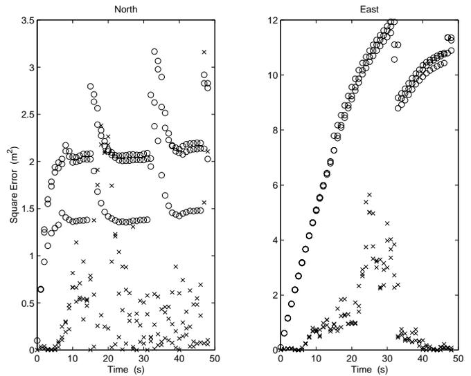
Figure 6: Estimated (circles) and actual (crosses) vehicle position squared error in the north and east directions. (This includes both projected and updated states.)
