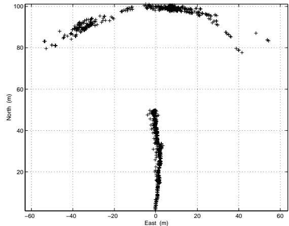
Figure 3: All vehicle and feature states for a simulated run with one feature. The vehicle starts out at (0,0) and moves north at 1 m/s. The feature is stationary at the location (100,0). 1954 total states are hypothesized, 747 are feature states and 1207 are vehicle states.
